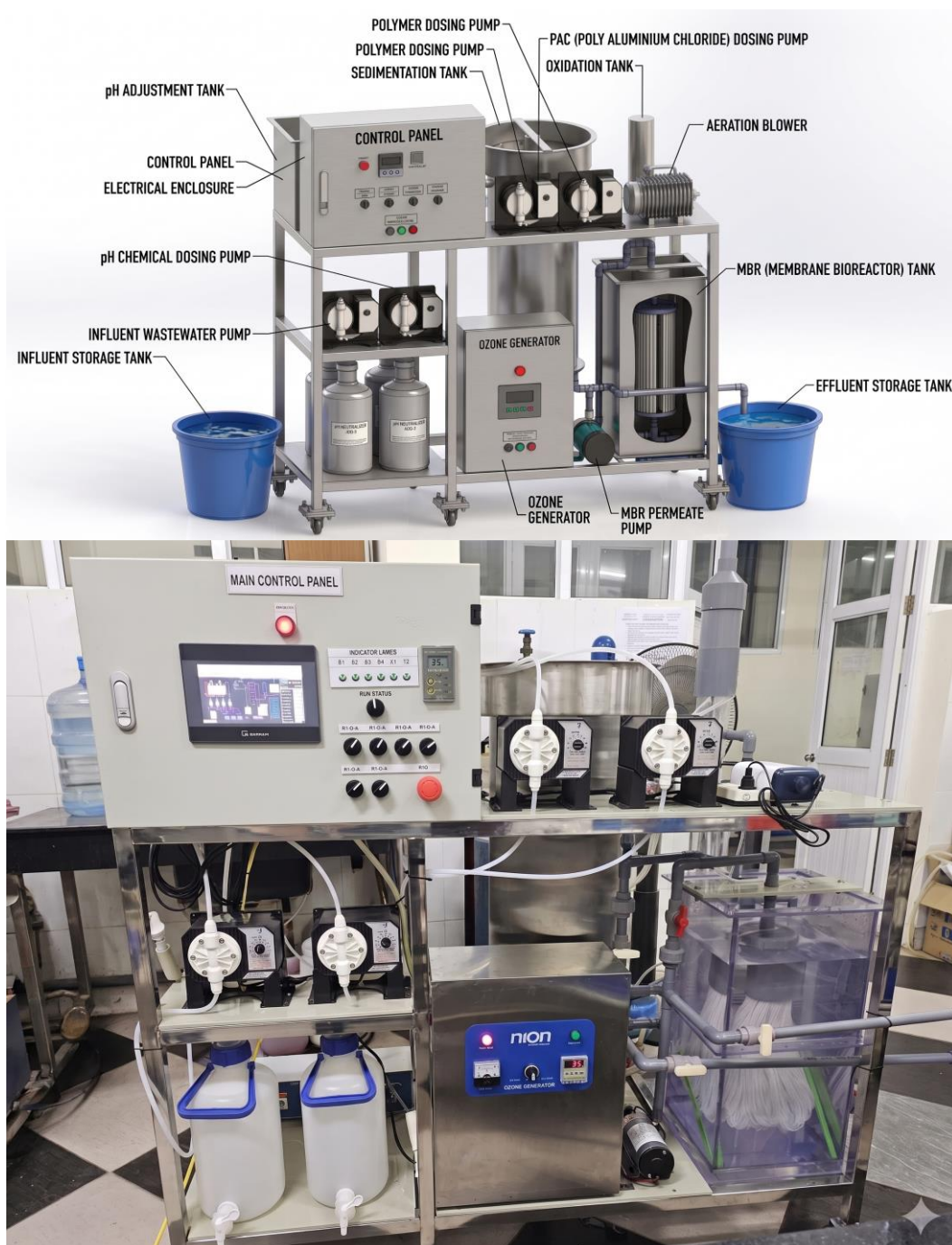
Figure 1 Schematic and experimental setup of the integrated laboratory-scale coagulation–sedimentation/ O_3 -AOP/MBR hybrid system for treating simulated pharmaceutical and resin synthesis wastewater.
