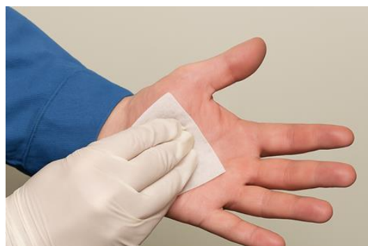
Figure 1 Illustration of hand wipe sampling using wash hand wipes for heavy metal analysis.
