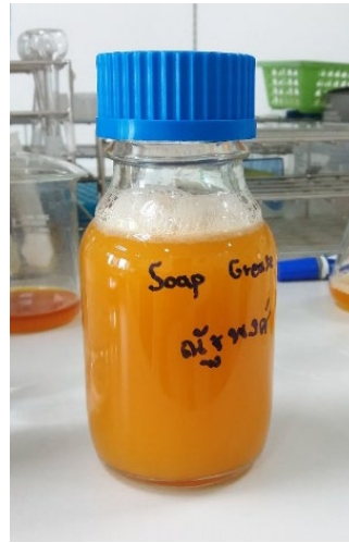
Figure S2 Grease trap soap produced under Optimal A condition at the processing time of 3 hours.
