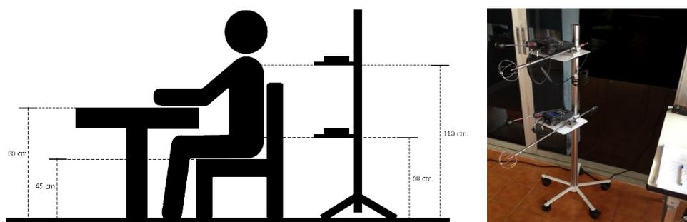
**Figure 1** The instrument installed with the Kimo AQ300 at two heights (0.6 m and 1.1 m).
