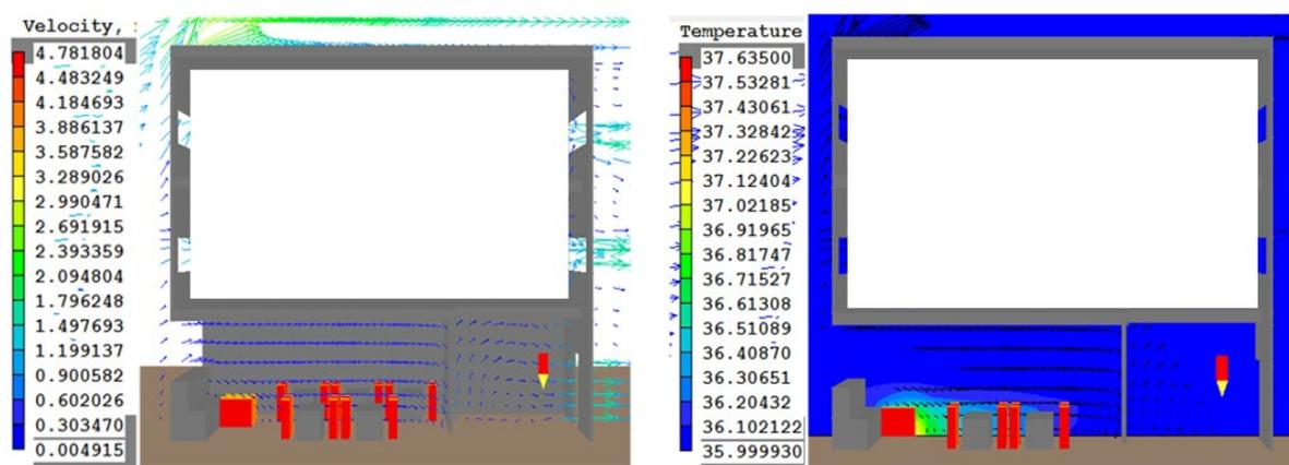
**Figure 3** Simulated temperature ( $^{\circ}\text{C}$ ) and airflow velocity ( $\text{m s}^{-1}$ ) results in the first row house/restaurant combination.
