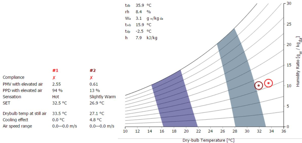
**Figure 7** Comparison of conditions in the second restaurant: initial measurement (purple) and increased ventilation with the adjusted humidity techniques (grey).
