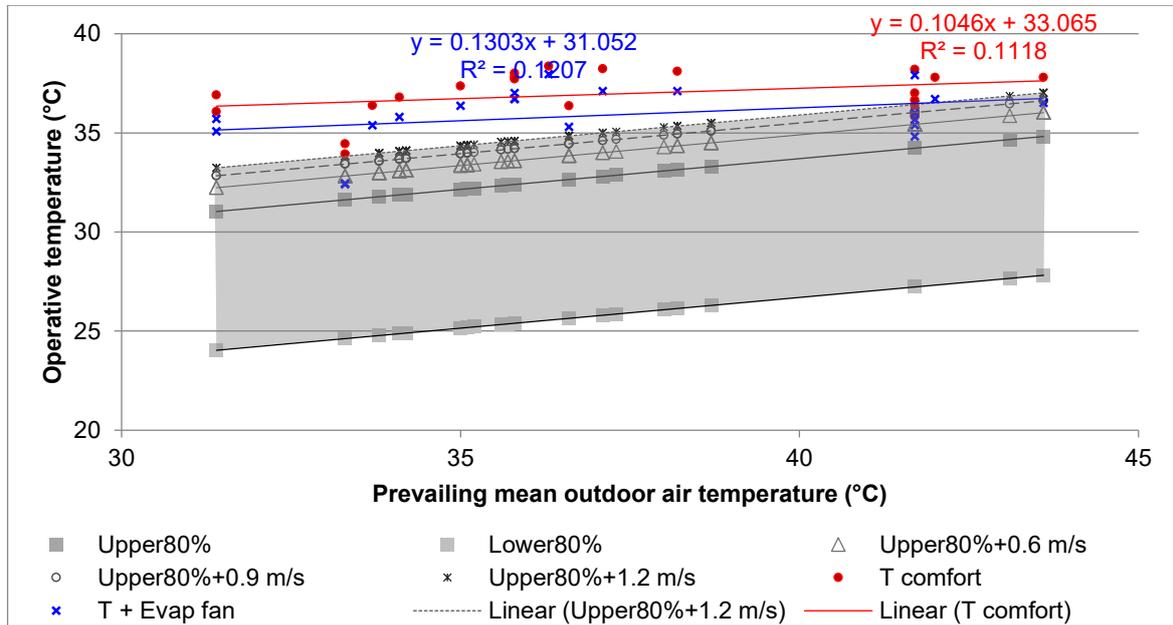
**Figure 4** Comfortable temperature in the acceptable operative temperature ranges for naturally conditioned spaces (from the first restaurant).
