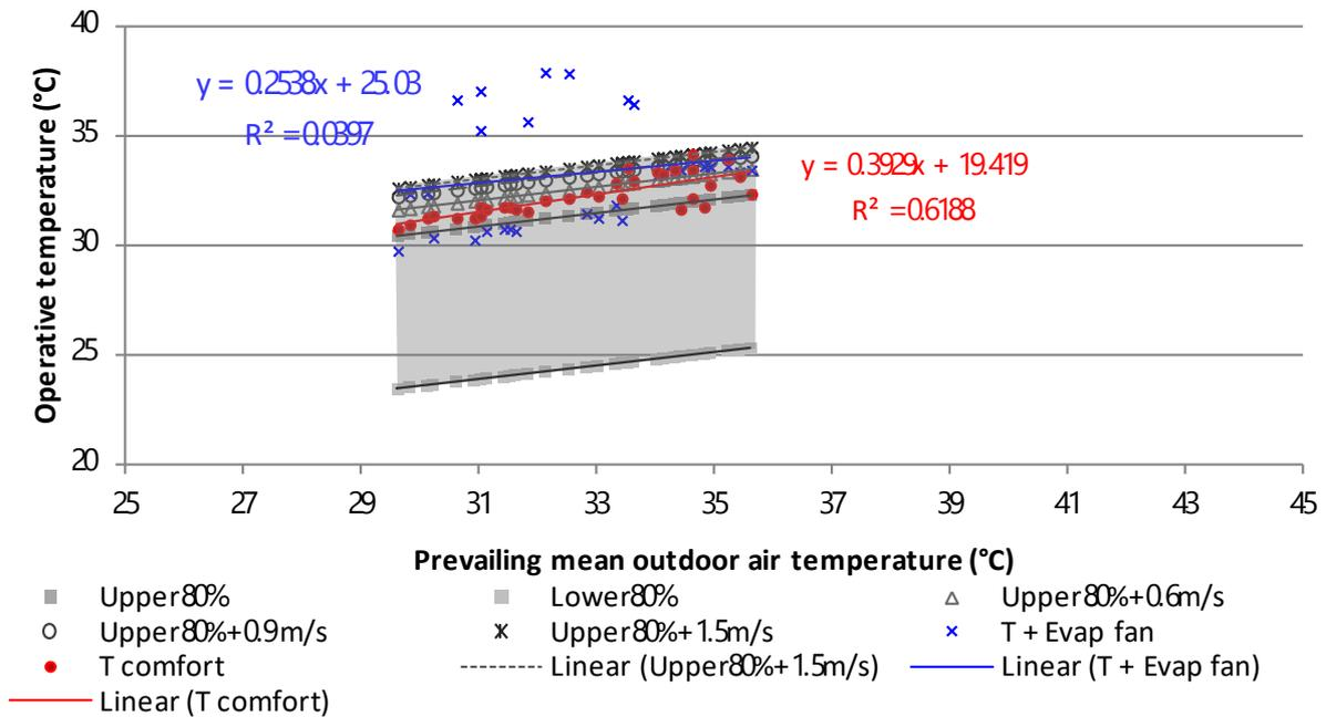
**Figure 5** Comfortable temperature in the acceptable operative temperature ranges for naturally conditioned spaces (from the second restaurant).
