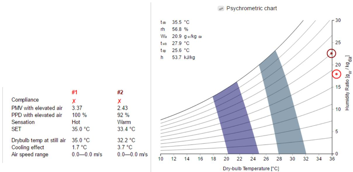
**Figure 6** Comparison of conditions in the first restaurant: initial measurement (purple) and increased ventilation with the adjusted humidity techniques (grey).
