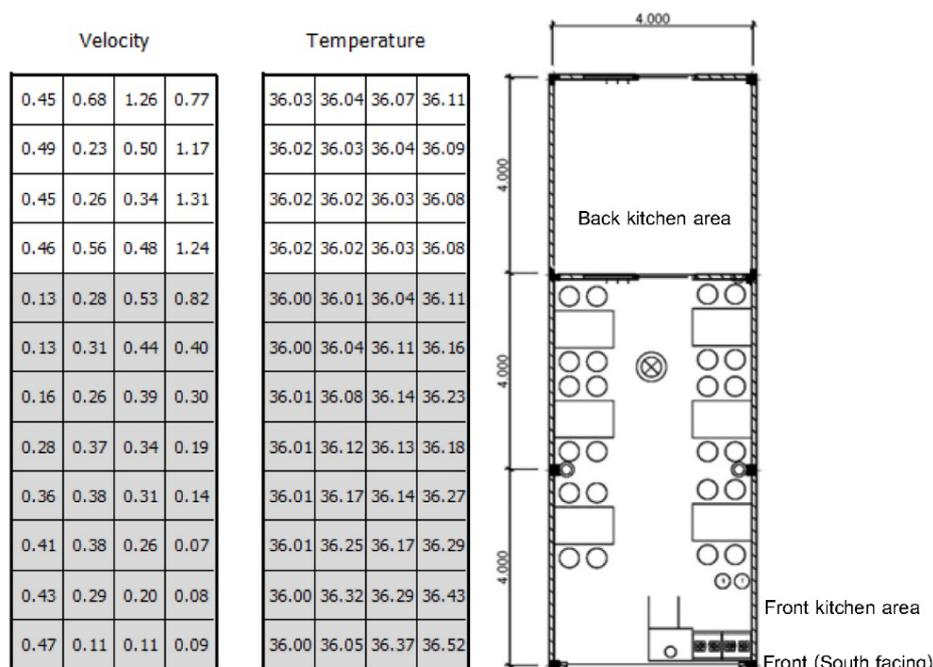
**Figure 2** Simulation results of the restaurant during full operation, presenting air velocity (m s<sup>-1</sup>) and temperature (°C).
