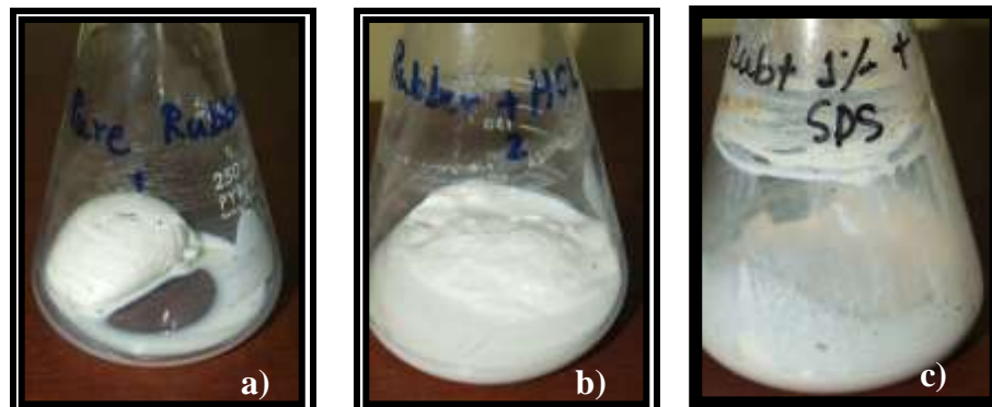
Figure 4 Destabilization and coagulation of latex particles (a) field latex b) field latex with pH adjustment and c) field latex with 1% of SDS addition)
