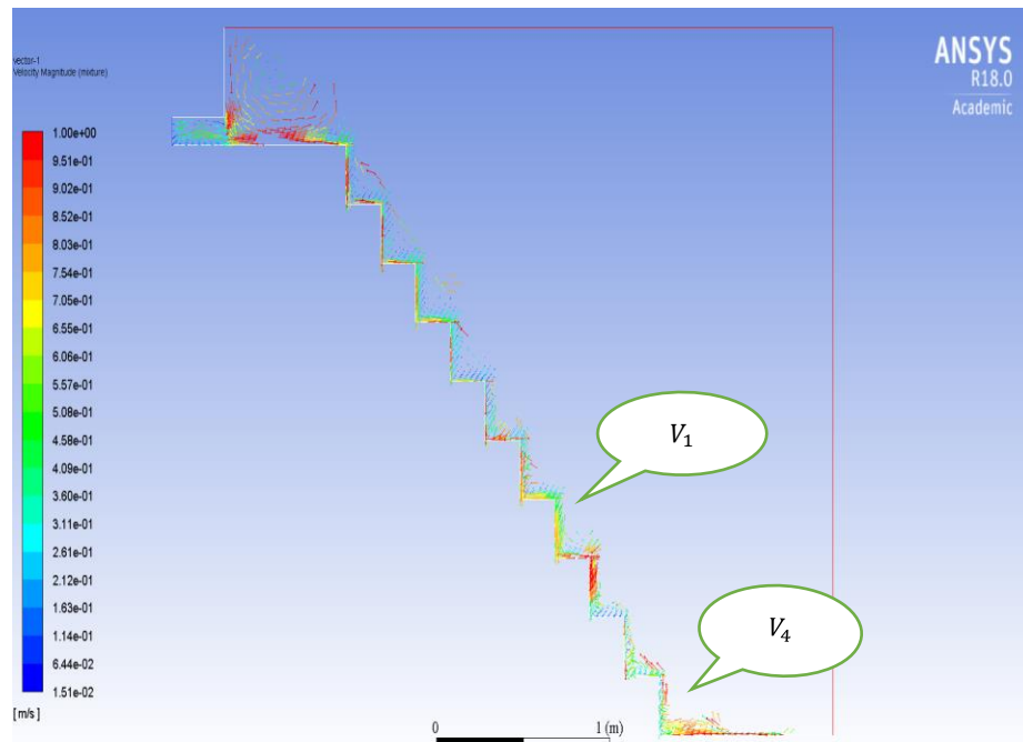
Fig. 15. Velocity on the numerical model at Q_1 = 4.21 \times 10^{-4} \text{ m}^3/\text{s} .
