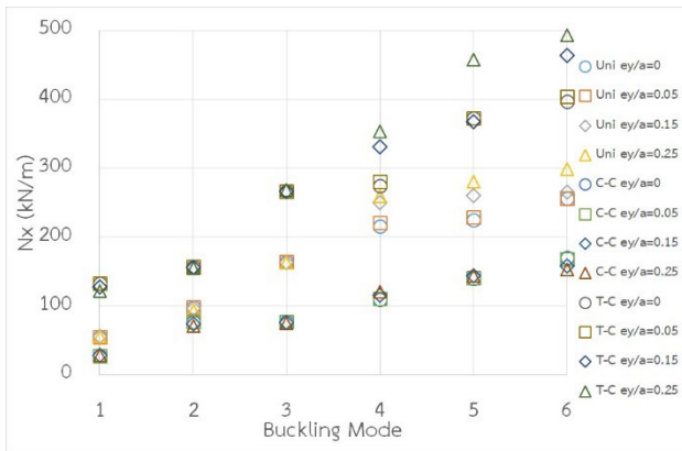
Figure 11: Buckling mode of plates with eccentric cutouts in y-direction at d/b = 0.2 subject to three loadings
