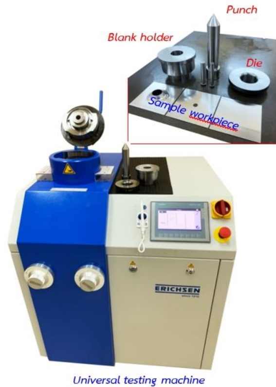
Figure 4: Hole flanging apparatus
