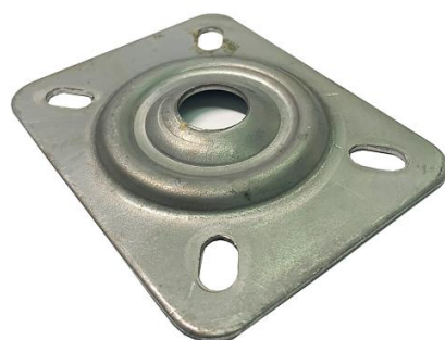
(c) Hole flanging application Figure 1: Hole flanging application
