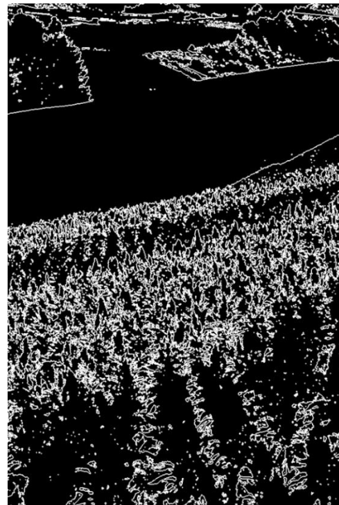
Figure 9: The edge between low intensity and high intensity areas of segmented image in Figure 6.
