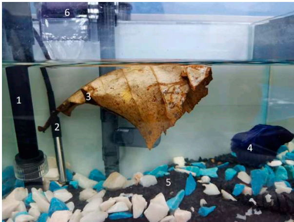
Figure 4 Internal Aquarium Setup. 1. pH sensor, 2. Water temperature sensor, 3. Indian Almond leaf, 4. Betta Fish, 5. Coarse gravel and marble base and 6. External hanging filter coupled with surface skimmer.
