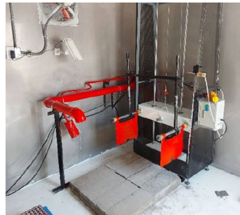
Figure 11: Impact battery test chamber
