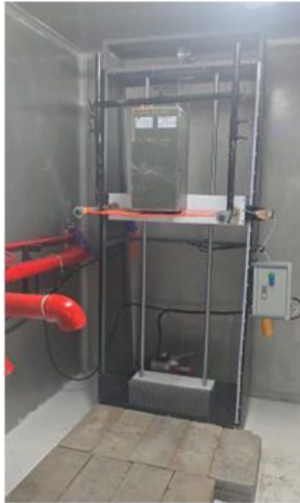
Figure 12: Battery drop test in case of S5 position
