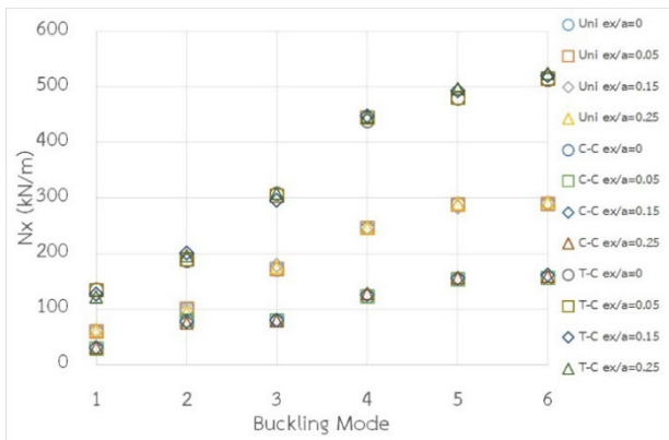
Figure 7: Buckling mode of plates with eccentric cutouts in x-direction at d/b = 0.1 subject to three loadings
