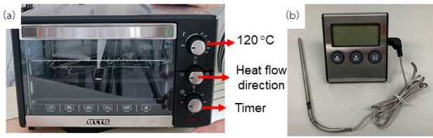
Figure 1: Equipment used for the VBO process used in this study: (a) Toaster oven and (b) temperature sensor.
