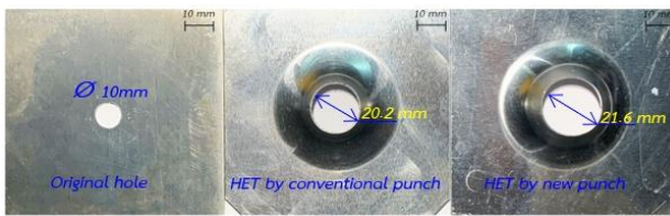
(a) Sample of hole expansion of AA1100
