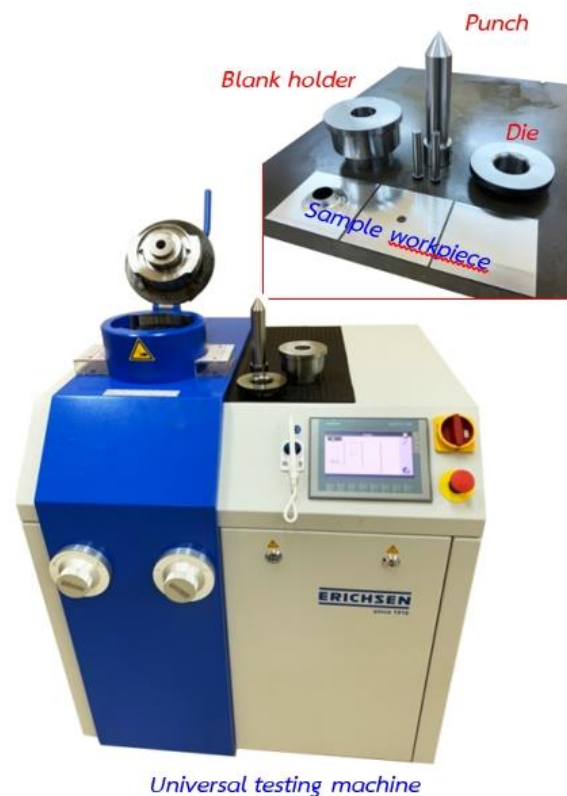
Figure 4: Hole flanging apparatus
