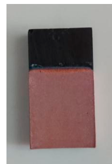
Figure 4 Sample of copper electroplated graphite electrode
