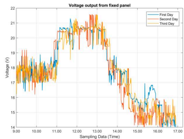
Fig. 12 voltage output from fixed panel
