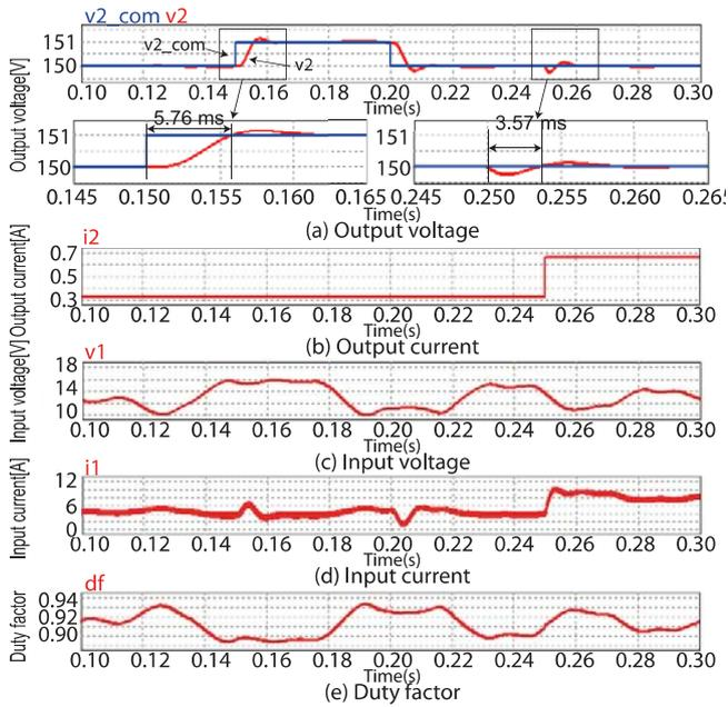
Fig. 7 The adaptive ILQ control with the stable photovoltaic generation (The input voltage  $v_1$  is similar to the output of photovoltaic battery)
