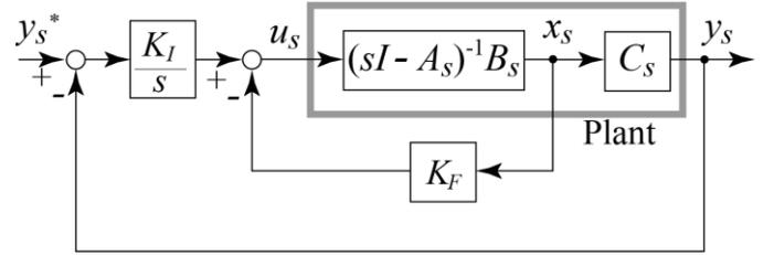
Fig. 3 Block diagram of typical servo-system
