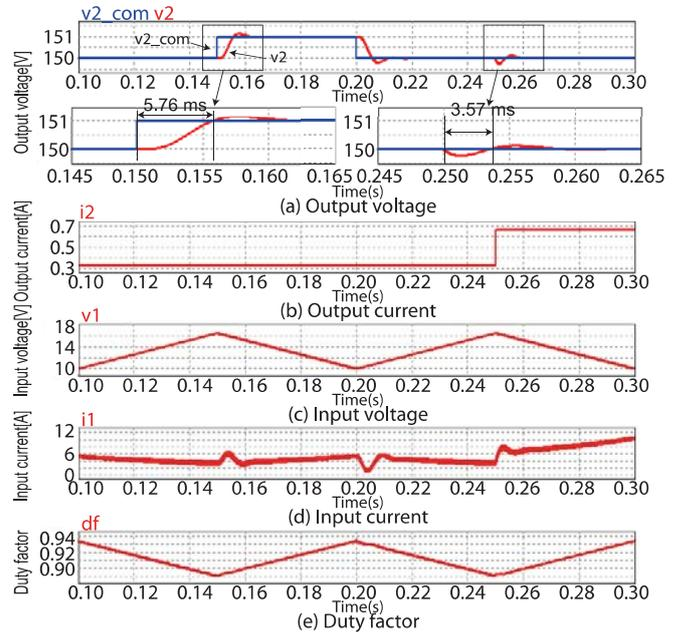
Fig. 6 The adaptive ILQ control with the stable photovoltaic generation (the input voltage  $v_1$  changes triangle waveform)
