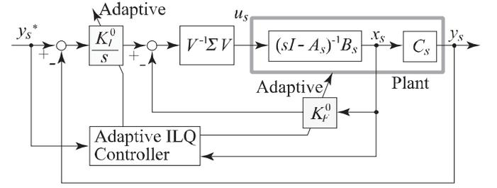
Fig. 5 Block diagram of construction of the adaptive ILQ servo-system for the stable photovoltaic generation by boost converter
