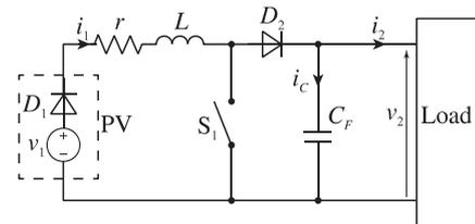
Fig. 2 Equivalent circuit of the boost converter
