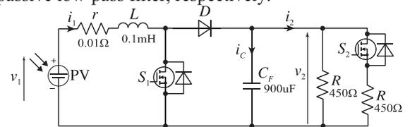
Fig. 1 The boost converter circuit
