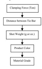
Fig. 1 Injection molding machine selection criteria
