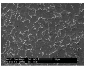
Fig. 7 SEM micrograph of the mold, showing grain in the electrode area Grain size is a critical parameter to characterize the microstructure, as it is strongly related to mechanical properties. Since strength increases with decreasing grain size, excessive grain growth should be avoided to prevent deterioration of mechanical properties.
