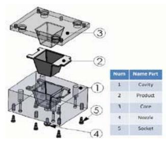
Fig. 1 Schematic presentation of compression mold, showing cavity part, rubber product, and core part designated with #1, 2 and 3, respectively
