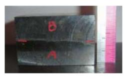
Fig. 2 Cross section of core part of the mold, showing substrate and deposited electrode, designated as region A and B, respectively
