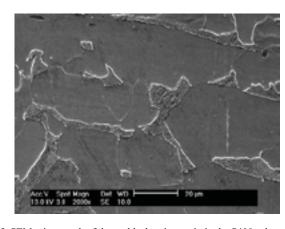
Fig. 5 SEM micrograph of the mold, showing grain in the S400 substrate area
