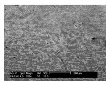
Fig. 4 SEM micrograph of the mold showing small pores in the sample
