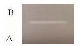
Fig. 3 Radiographic image of core part of the mold, showing substrate and deposited electrode, designated as region A and B, respectively
