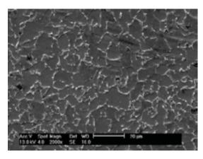
Fig. 6 SEM micrograph of the mold, showing grain in the interface area
