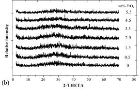
Fig. 1 The XRD patterns of ZIG glasses containing  $ZrO_2$  in the range of 0-5.5 wt% after melted at (a) 900 °C and (b) 1000 °C
