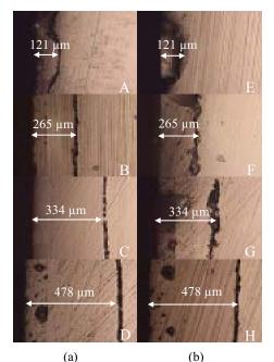
Fig. 4 The optical micrographs of 5.5CGS after coated with 5.5ZIG melted at (a) 900  $^{\circ}$ C (A-D) and (b) 1000  $^{\circ}$ C (E-H)
