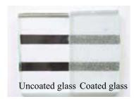
Fig. 2 Uncoated and coated glass sheets by using 5.5ZIG coating glass
