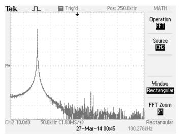
Fig. 7. Illustration of the Fast Fourier Transform for THD calculations.
