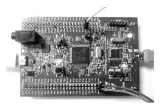
Fig. 4. The photograph of the utilised STM32F4 microcontroller as an interface device for A/D converter.
