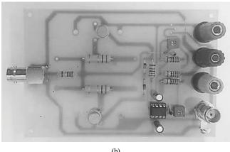
Fig. 3. The preamplfier circuit designs; (a) circuit diagram, (b) circuit implemenation on board.
