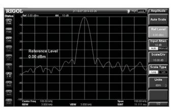
Fig. 8. Illustrations of the power spectral density showing the bandwith of the signal at 0dBm level.
