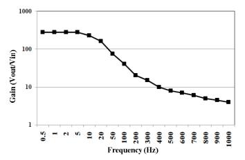
Fig. 5. Frequency characteristics of the proposed preamplifier
