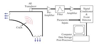
Fig. 1. Typical acoustic emission sensor detection system.
