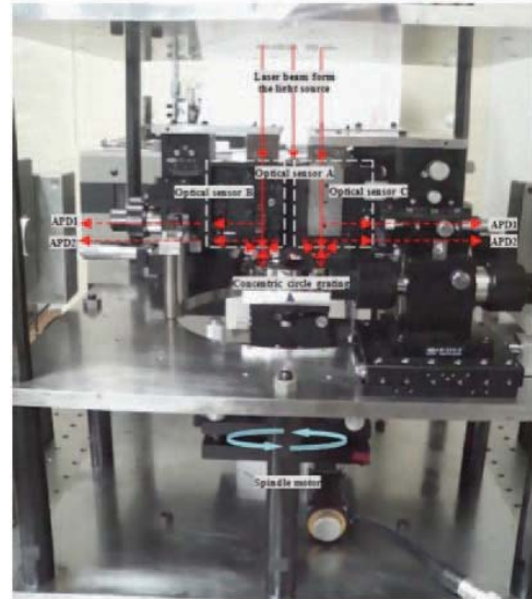
Figure 3 Measurement system for spindle radial, axial and angular motions
