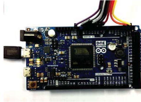
Fig.6 Arduino with Atmel SAM3X8E ARM Cortex-M3 CPU
