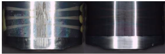
(a) Al_2O_3 protection film (b) DLC protection film
