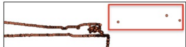
Fig. 9 Jumping GPS points (in the box)
