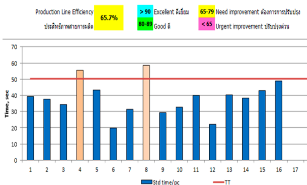
Fig. 2 The Yamazumi Chart of the side airbag sewing process
