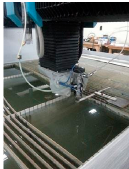
Fig. 1 shows a typical layout of an abrasive waterjet machine.
