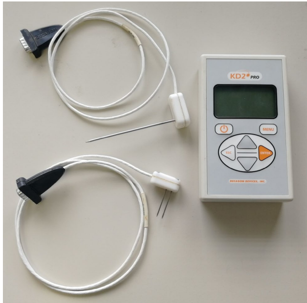
Figure 1 KD2 Pro Thermal Properties Analyzer (Source: Geological Survey of Slovenia [GeoZS], 2025).
