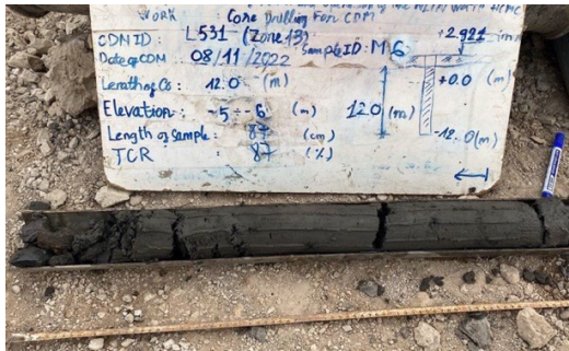
(a) A core sample taken in the L531 column in Zone 13
