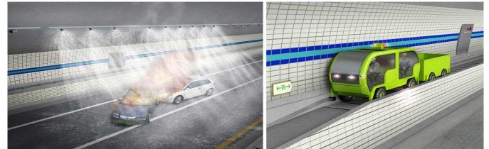
Figure 31 Water-mist fire extinguishing system and maintenance vehicle moving on the conduit
