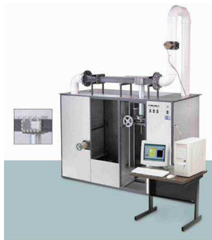
Figure 1. Erosion Function Apparatus to measure erodibility (Briaud et al., 1999)
