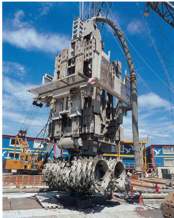
Figure 49. Two-axes rotating type cutting bits
