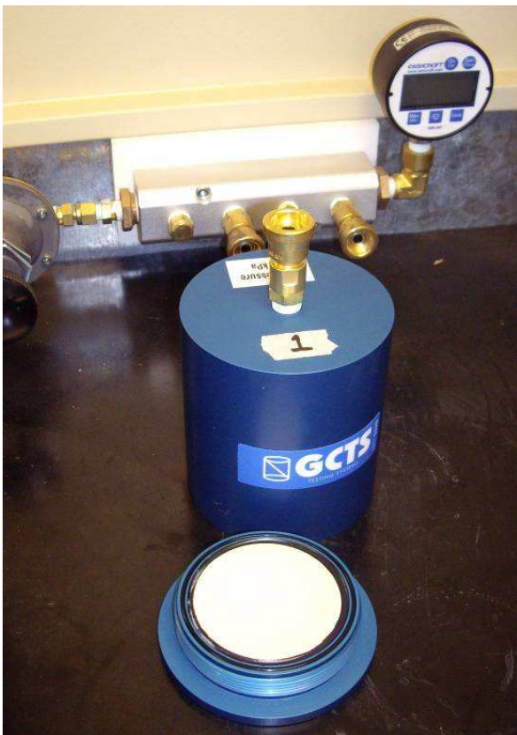
Figure 6. Pressure Plate Apparatus used at Golder Associates (Saskatoon) for the measurement of the Soil-Water Characteristic Curve, SWCC
