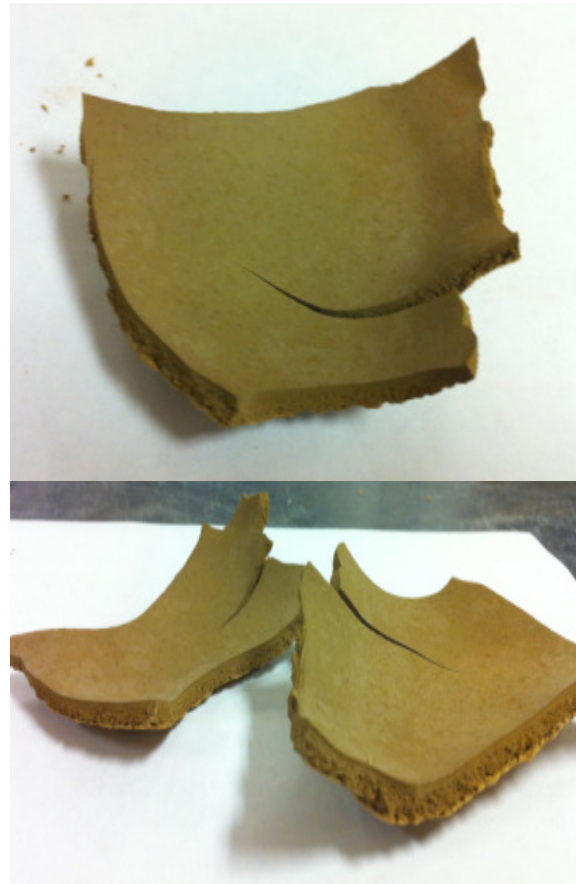
a) Soil curling at the edges (irregular pattern)
