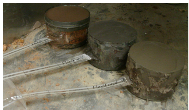
Figure 6 SIP test in horizontal orientation (SIPH)
