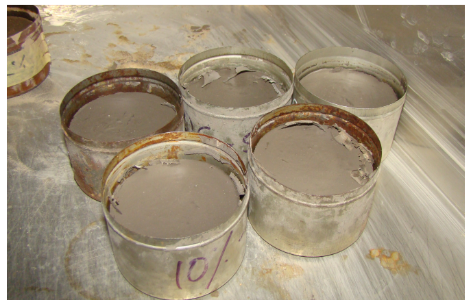
Figure 10 Dry soil specimens used in IDT testing
