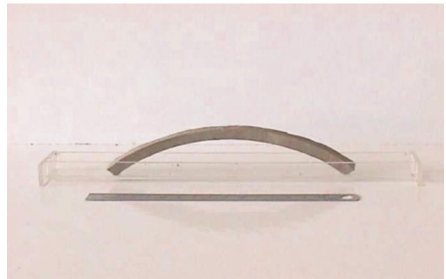
b) Curling of soft Werribee clay (ideal pattern) (Kodikara et al, 2004)
