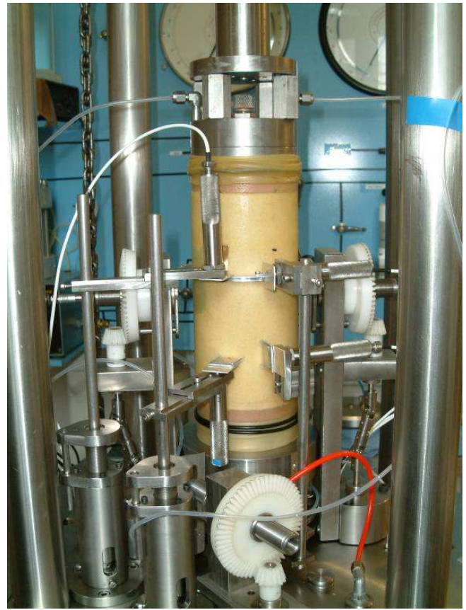
Figure 2 Local small strain measurement systems.
