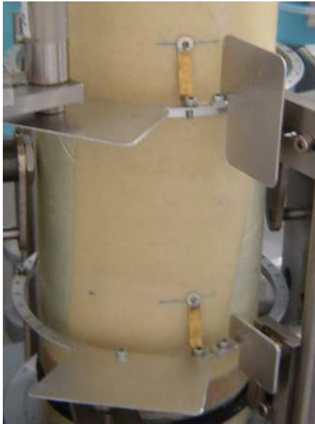
Figure 7 Aluminum targets fixed on two rings located on the central part of the specimen (top and bottom); the flexible suspension connections are glued on the outer membrane
