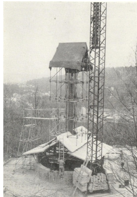
Figure 3 Facility developed at Iraba to test models of deep foundations and penetrometers (Kérisel, 1961)
