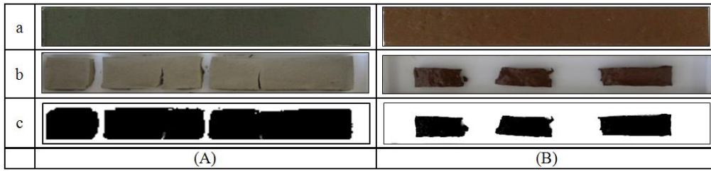
Figure 3 Linear shrinkage bar test (A) Bangkok clay, (B) Bentonite (a = before air-dried, b = after air-dried, c = binarised to black and white after image thresholding on air-dried specimens)
