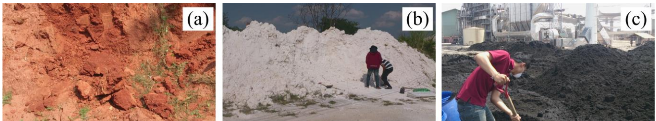
Figure 1 Raw materials of the study; (a) red loess, (b) MDW, and (c) SBAW
