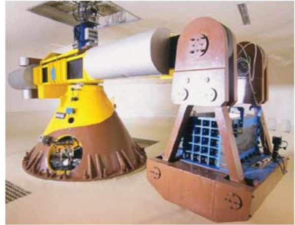
Figure 3 View of a 4.5 m radius large beam centrifuge facility at IIT Bombay
