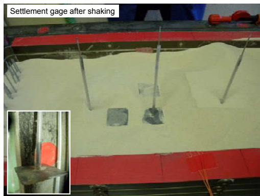
(c) Settlement gauges and PVC plates after the test
