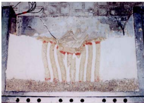
Figure 9 Failure mode of compacted sand piles (No.1)
