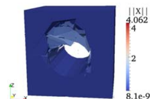
Figure 3 Failure of model due to the gravity fall of rock blocks at the 49 th time step (end of four excavation phases)
