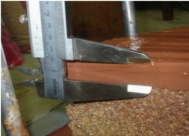
Figure 21 Photo of cake film from model test (Teparaksa, 2008)
