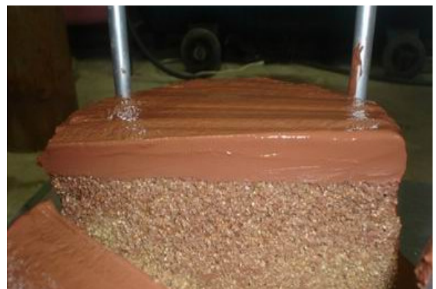
Figure 20 Photo of cake film from model test (Teparaksa, 2008)
