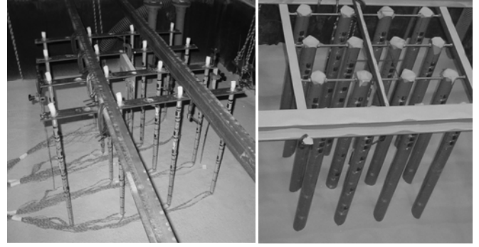
Photo 1 Model piles set-up prior to preparing model ground
