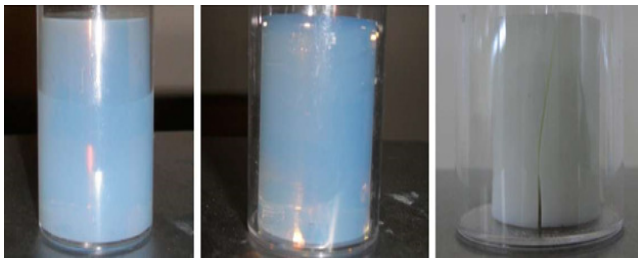
(a) Initial state; (b) Progressive volumetric shrinkage; (c) Cracks after 3 months
