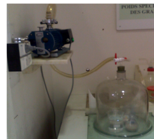
Figure 4 Drying chamber of 80°C and vacuum pump
