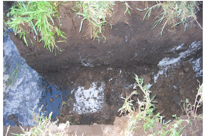
Figure 7 Lime-fly ash barrier at 1m below ground surface (after Banasiak (2004))
