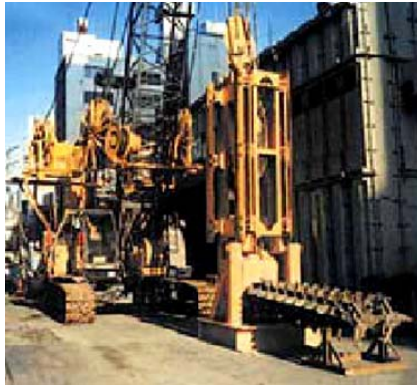
Figure 25 Excavation Machine under Existing Structure (SATT method) 29)
