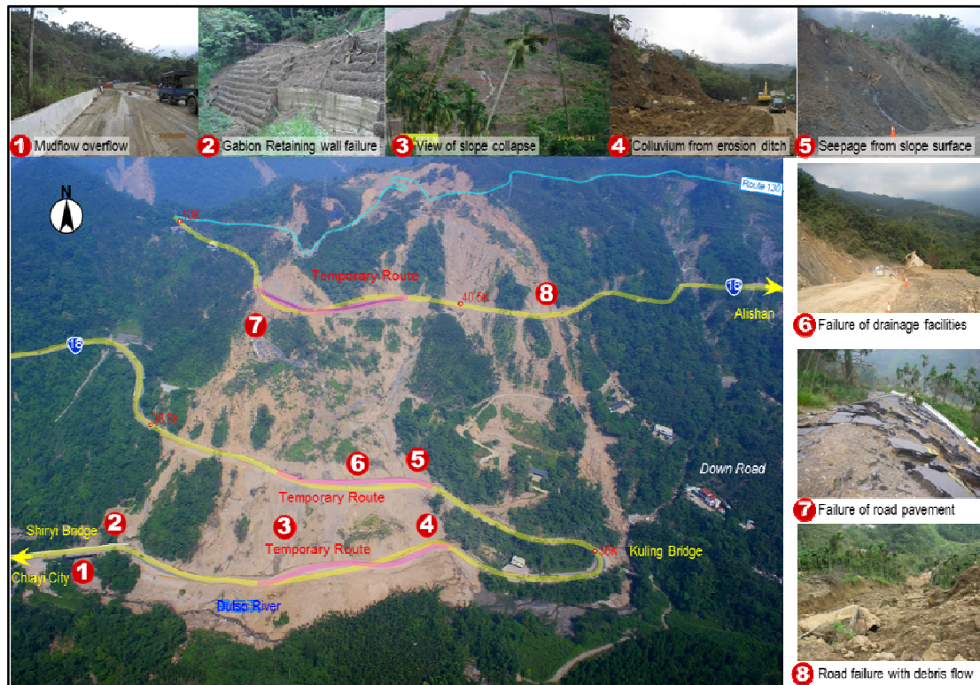
Figure 3 Slope slide disaster photos at mileage 37.5k
