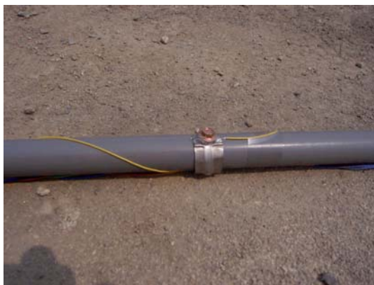
Figure 20 In-hole resistivity sensors for 3D RIP tests
