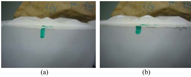
Photo 3 Failure pattern after joints are sheared with t/a=1 and w=50\% (a) \sigma_n=0.3\text{MPa} , (b) \sigma_n=1.0\text{MPa}
